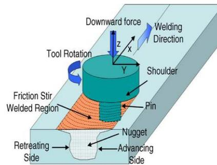
Fig. 1 Friction Stir Welding Schematic Set-up [10]
